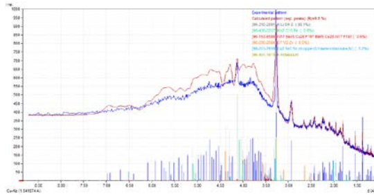
Fig. 3.1.2.1 (b) XRD pattern of MR dye untreated sargassum vulgare powder with matching compounds
