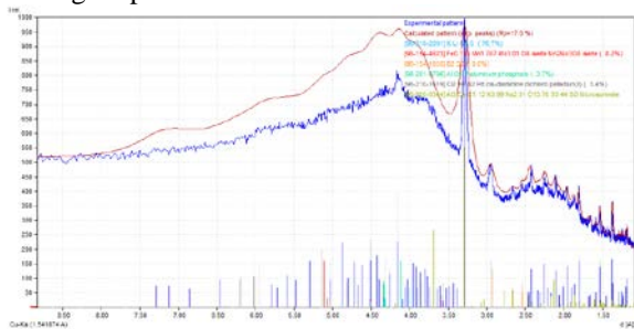
Fig. 3.1.2.2 (b) XRD pattern of MR dye treated Sargassum vulgare powder with matching compounds
